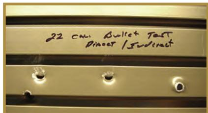
Figure 1: An aluminum metal sheet treated with ECOPHOR B/700 and then painted with epoxy polyester powder coating. After a cross-hatch adhesion test to verify the paint flexibility and resistance to bending and mechanical shock, the customer shot the panel with a .22-caliber bullet from 5 meters. You can see that the coating perfectly "follows" the hole left by the bullet.
