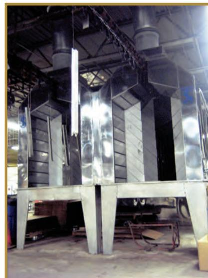
Figure 3: Dual in-line flowcoat tunnels for multi-shift production. Each tunnel is equipped with its own tank and filtering system. Specific risers can be turned on or off—depending on conveyor speed—to allow for appropriate treatment time and to minimize chemical consumption.
