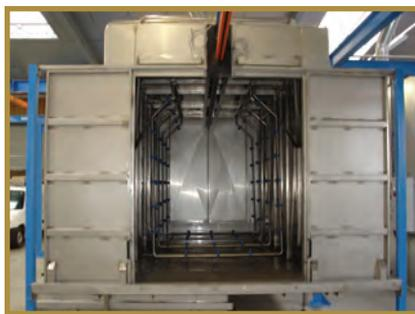
Figure 2: Manual batch spraying equipment. Parts are hung and manually placed in the washer. The unit is equipped with three risers with nozzles, and the risers—rather than the parts—move during treatment to completely bathe all the part surfaces.
